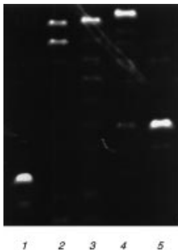
Fig. 1. Primer-extension assay of p 3 isoG d (1) with 2.5 U of Klenow fragment at 37° . Fluorescein-labeled primer I is extended in the presence of control template II and p 3 T (Lane 2). Primer I is elongated to full-length product in the presence of me 5 isoC d -containing template III , p 3 T, and either p 3 isoG d (Lane 3) or a substituted p 3 isoG d from a related work (Lane 4) [18], but not in the presence of only template III and p 3 T (Lane 5). Primer I alone is included for comparison (Lane 1).
